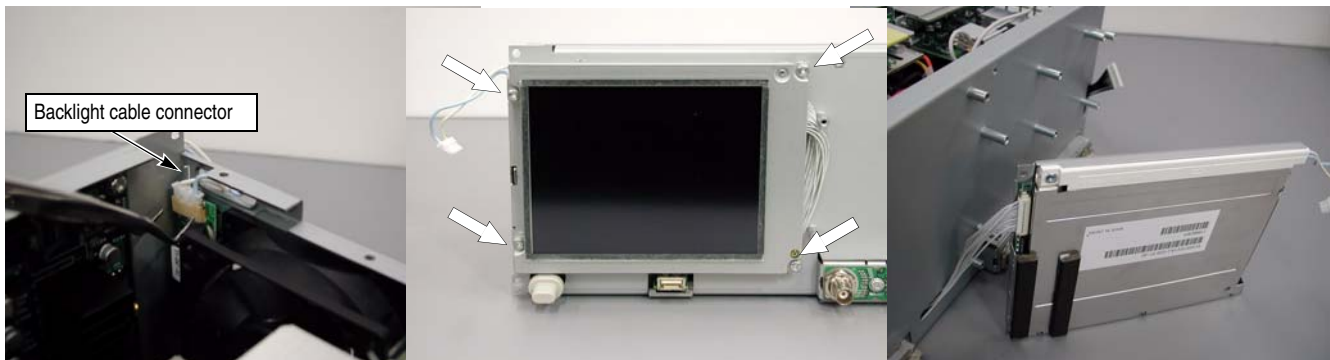
Figure 6-8: Display module removal
