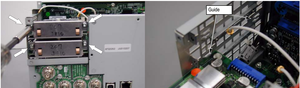
Figure 6-9: Output board removal
