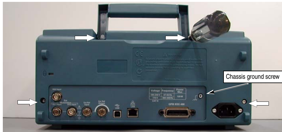
Figure 6-3: Rear case removal
