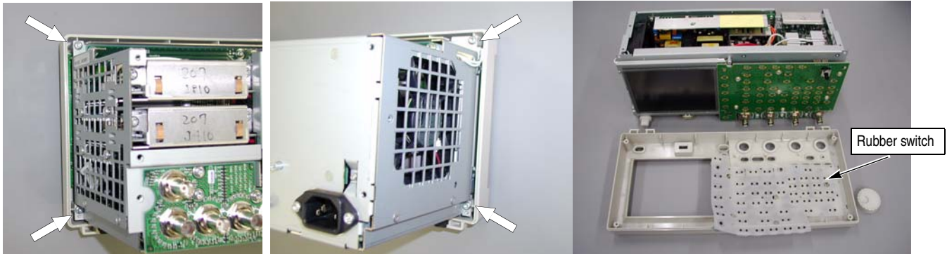
Figure 6-6: Front case removal
